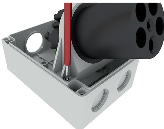
4. Open the contact slide (5) by forcing it with a screwdriver and pull the individual conductors from the terminals.
