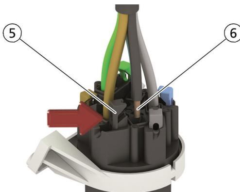
9. Check whether the individual conductors are seated tightly by pulling them lightly. If this is not the case, open the terminal and repeat the previous step.
